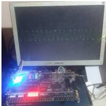
Figure 15. Experimental set-up of the FPGA-based implementation of ASK and QAM modulator using a DE2 115 board and the VGA Screen.
