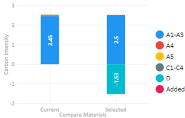
Figure 9. Material-based ECI variance for steel bar joist layer.
