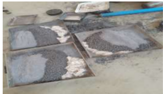
Figure 5. Soil-CHA and Enset fiber mix preparation.
