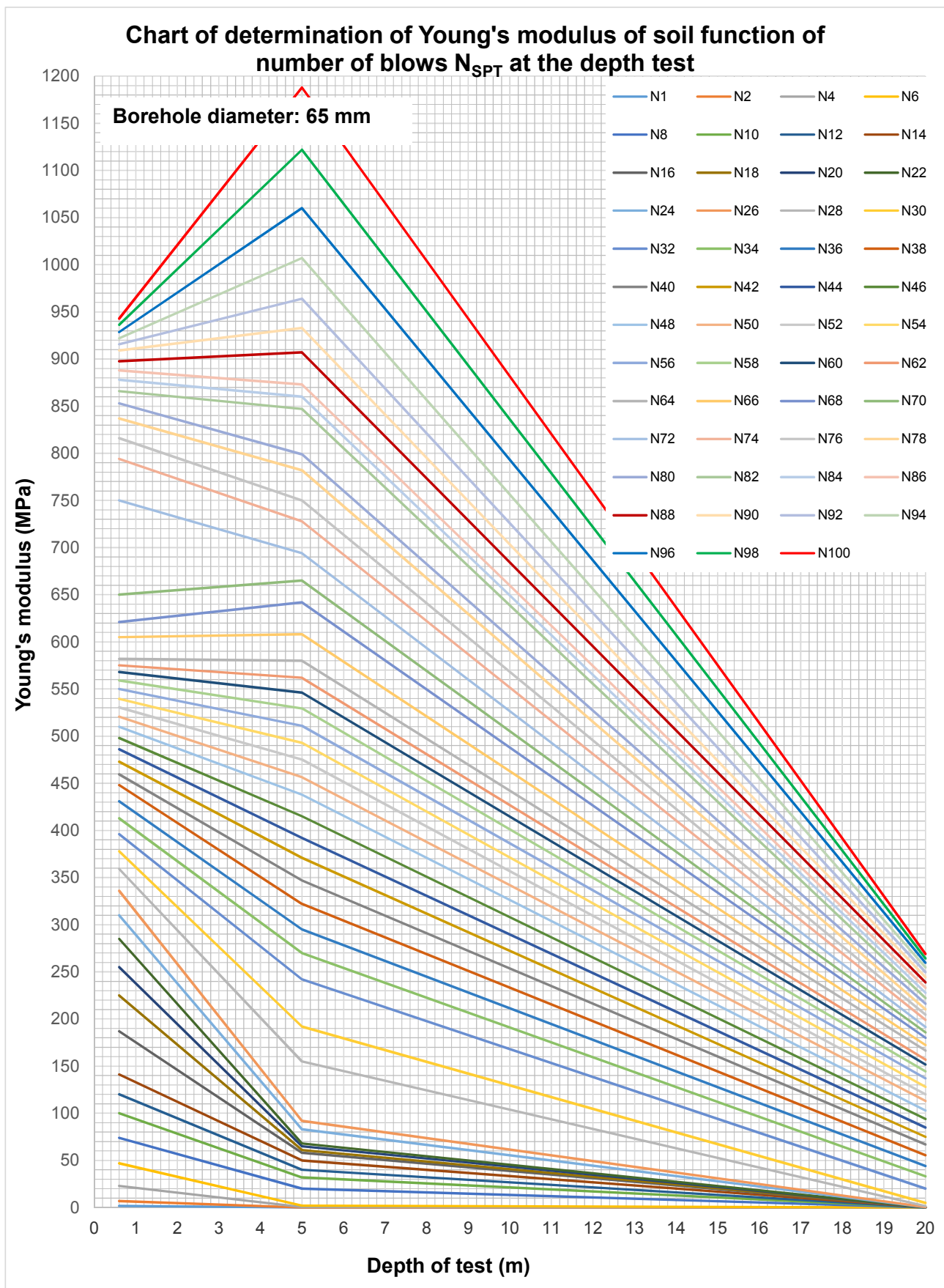
Figure 19. Young's modulus vs number of blows and depth of test (borehole diameter = 65 mm).
