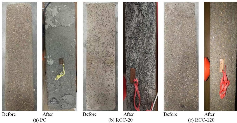
Figure 7. Appearance comparison of specimens before / after freeze-thaw test.
