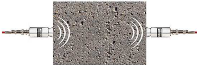
Figure 1. Plane ultrasonic transducers.
