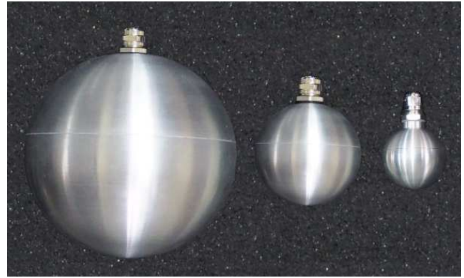
Figure 8. Spherical embedded ultrasonic transducer.
