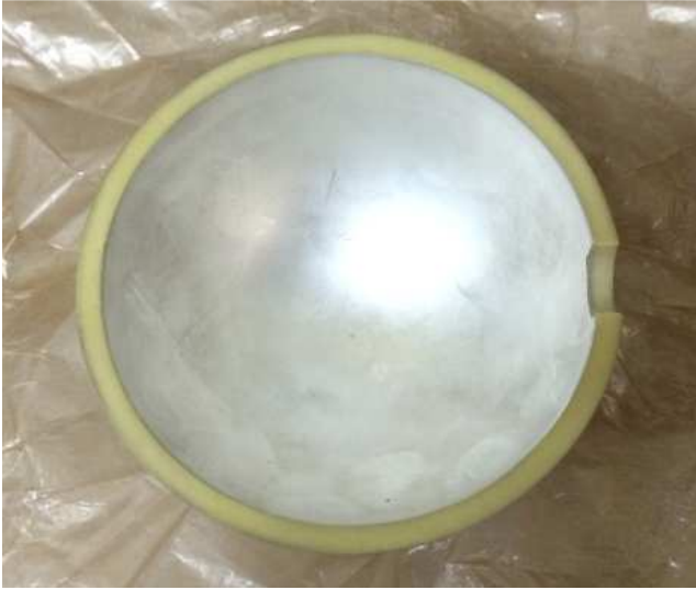
Figure 7. Hemisphere piezoelectric ceramic crystal.
