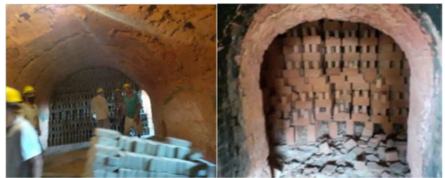
Figure 5. (a), (b): Position of bricks inside the kilns.
