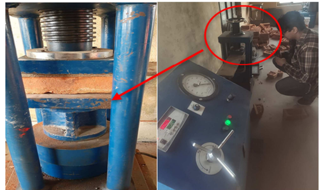
Figure 9. Compressive Strength Test of Brick Samples.
